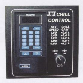
Precise chill roll "gain" control is essential to minimize cut-to-print variation and for overall web stability. All JII Outfeed Chill Roll Systems feature a Digital Speed Controller (Shown Above) coupled with a rugged precision Harmonic Drive Transmission System (Show Below) to ensure accurate web speed control.
