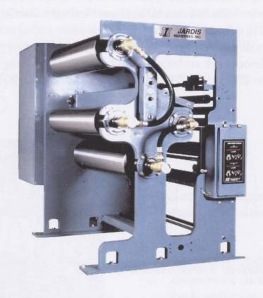
Jardis Industries' Outfeed Chill Roll Systems provide rugged, reliable web cooling and speed regulation essential for high quality heat-set web printing.
